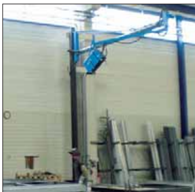
■ « ERGOMIG 2D » booms with a working radius of 2.6, 3.6 or 4.6 m
