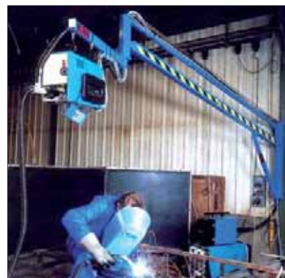
■ « AEROMIG 3D » booms with adjustable parallelograms and a working radius of 2.6, 3.6 or 4.6 m
