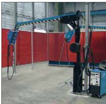
■ « GIRAFE » booms with a working radius of 2.5 or 3.5 m
