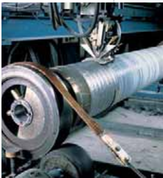
Hard-surfacing of mill rolls with strip cladding
